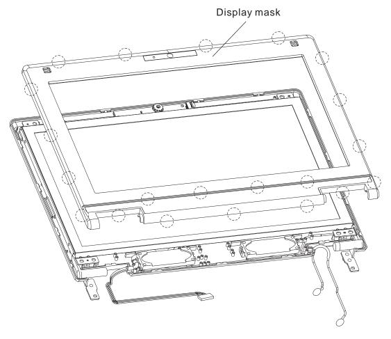
Figure 4-18 Removing the display mask
